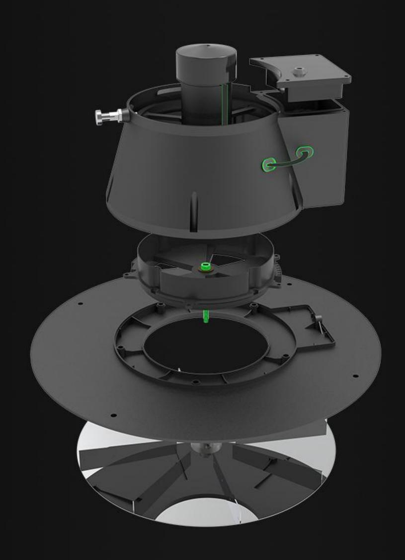
The new version spreader adopts upper and lower segmented drive shaft design. Screws are screwed externally, so won't stick fertilizers and can be easily disassembled and assembled from outside. The motor wiring is external to prevent fertilizers and liquids from entering the electric control hatch
