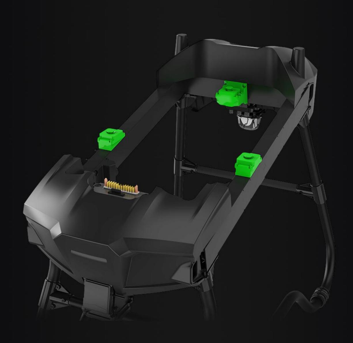
Weight sensor real-time remaining pesticide monitoring
